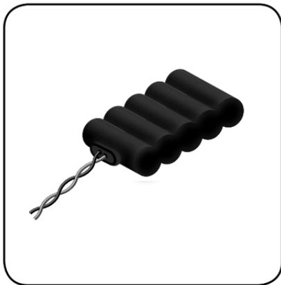
The battery pack is already in the battery compartment. Once you've set up the equipment and connected the battery, **you need to charge the pack for 16 hours initially.**
